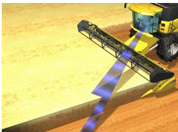
Rys. 5.31 System Smart Steer w kombajnach New Holland.
